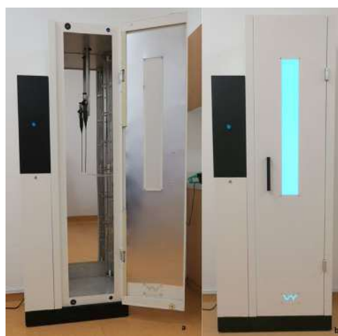
Fig. 1 a Arrangement of a FE in the D60. b Sealed D60 while reprocessing a FE
