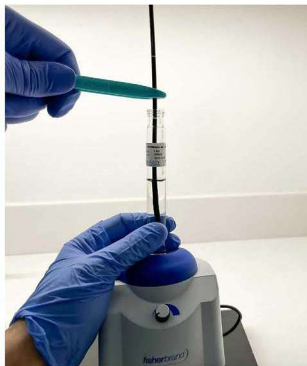
Fig. 2. Sample collection from the flexible fiberoptic laryngoscope (FFL) distal tip surface using vortex and collection tube. [Color figure can be viewed in the online issue, which is available at www.laryngoscope.com .]
