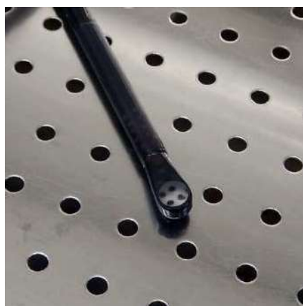
Figure 4. Dried inoculum on the tip of a TEE probe
